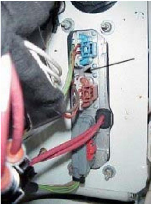
**Figure 93 Location: ESC on Engine Compartment Side**
