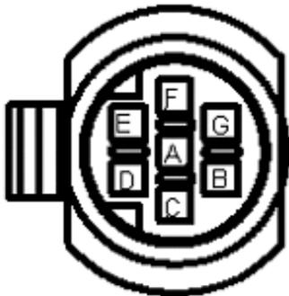
Connector on chassis harness viewed from mating end. This harness is located behind the driver's side headlight under the hood.
