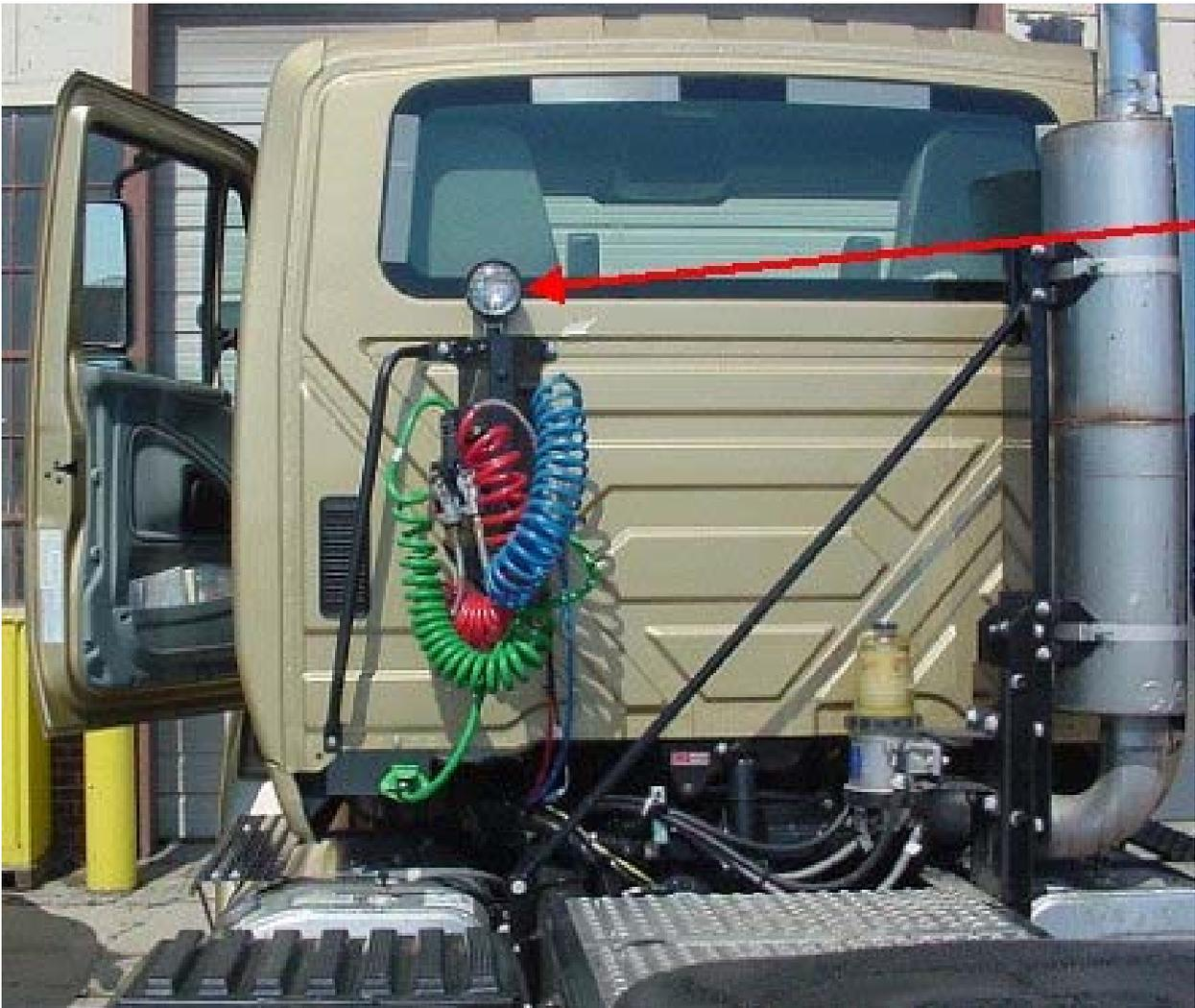
**Figure 81 Arrow Indicates Location of Work Light (Tractor)**
