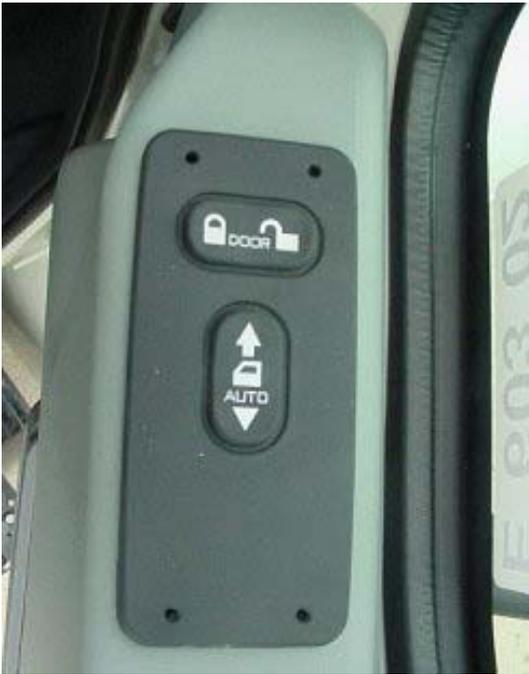
**Figure 98 Passenger's Side Door Pod**
